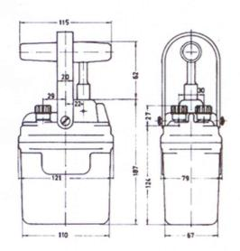
All electrical parts and the complete blasting machine are tested with a tension of 2000 V A.C.
